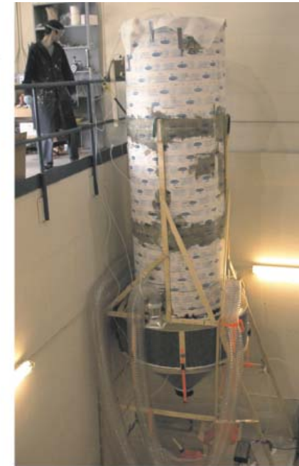
CO 2 absorption in prototype contactor [NaOH] = 1.3M, mean drop diameter = 175 μm
